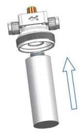
4.Use the matching wrench to tighten the upper cover nut
